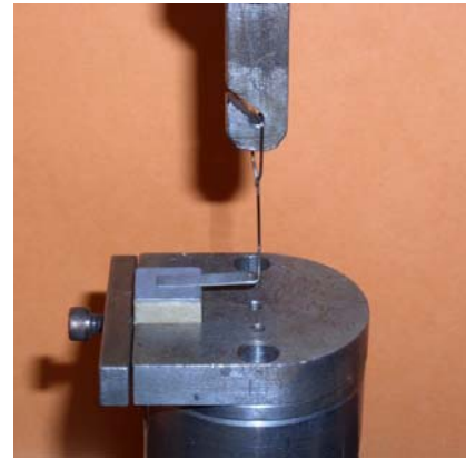
Fig. 2: The sample mounted in the Lloyd tensile machine during the pull out test.
