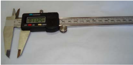
Fig. 1: Fowler Electronic Digital Calliper used in the measurements.
